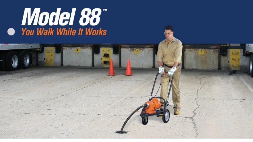
This machine is almost as easy to run as a lawn mower. You push eight or ten foot cable sections into the line until you reach some resistance. Then attach the rear cable coupling to the machine, stand behind it, and turn it on. Watch the cable feed itself into the line. When a section has run into the drain, attach another one and keep going. This self-feeding feature also works to pull sections out of the line.
